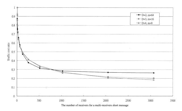
Fig. 22. The average multicast-to-unicast traffic cost ratio versus the number of receivers for a multireceivers short message for a 4096-node network for different values of SB size—m—and number of digits—D.
