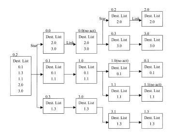
Fig. 12. A multidestination multicast routing example.
