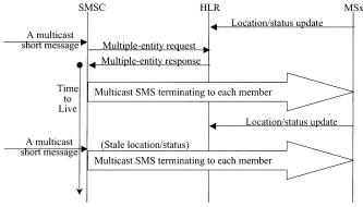
Fig. 9. Polling with piggybacked adaptive TTL approach for group member status and location tracking.
