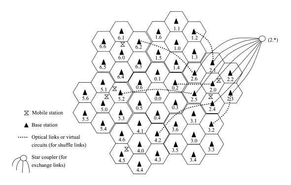
Fig. 1. Constructing the optical network from SBs.
