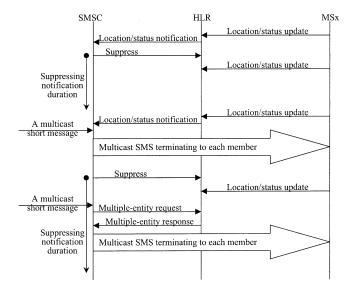
Fig. 11. Status update oriented with suppressing notification duration approach for group member status and location tracking.
